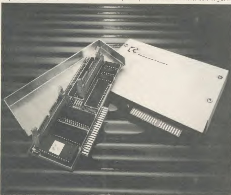
Cumana's Electron interface: plugs into the Plus1 and can support any format of disc drive
